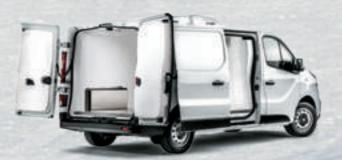
Vehicle with isothermal insulation, ATP approved, which can keep internal temperatures constant up to 0°C. If a refrigerating unit is installed, the compartment turns into a cold room that can transport medicines or food products.
