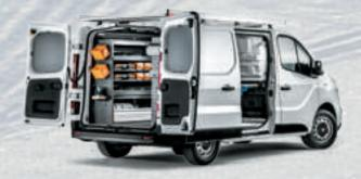
Version made of galvannealled automotive steel with modular and flexible quick fastening system.
